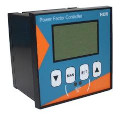
Automatic power factor controllers with microprocessor designed for signal processing of strongly distorted waveform to ensure accurate control of the electrical parameters of the plant. All measurements are made starting from the analysis of the waveform using FFT (Fast Fourier Transform) algoritm in floating point to ensure the maximum precision.
