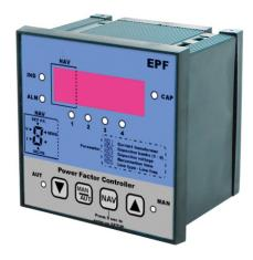
The power factor controller was designed with signal processing technology to ensure accurate control of all the electrical systems of the plant such as: VOLTAGE, CURRENT, COS $\phi$ , THD I% and through a sofisticate algorithm, optimal use of capacitors bank and contactors, taking into account the distortion phenomena of industrial plants.
